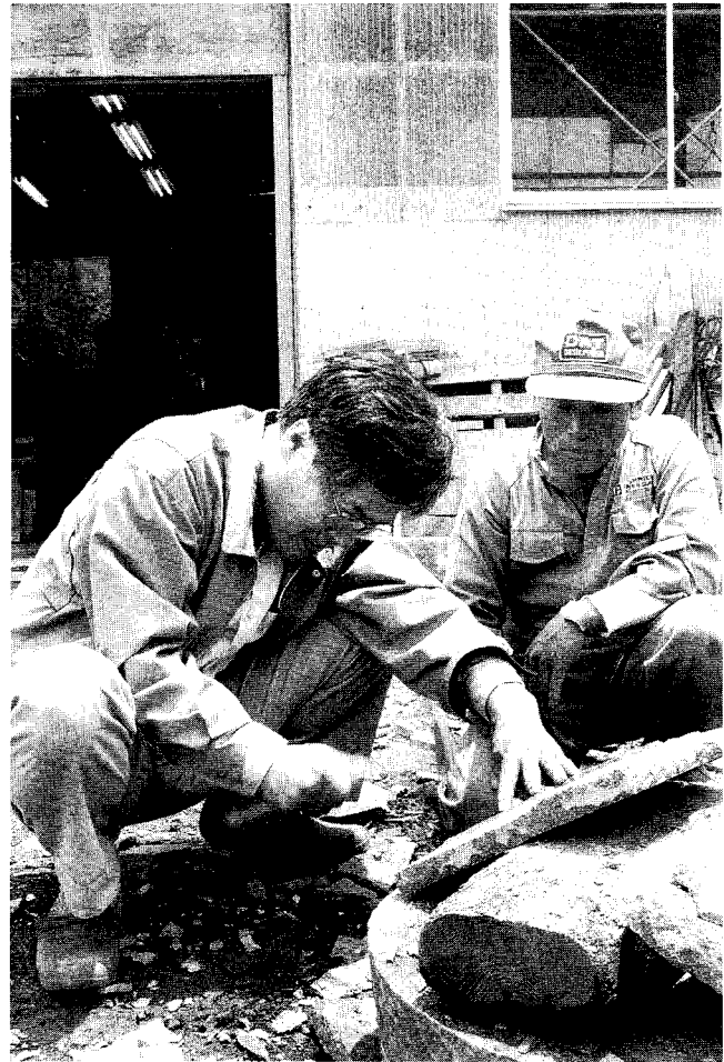
Fig. 4. Fujimori and Kitazawa experiment with creating a rough edge to tepei shingles.
